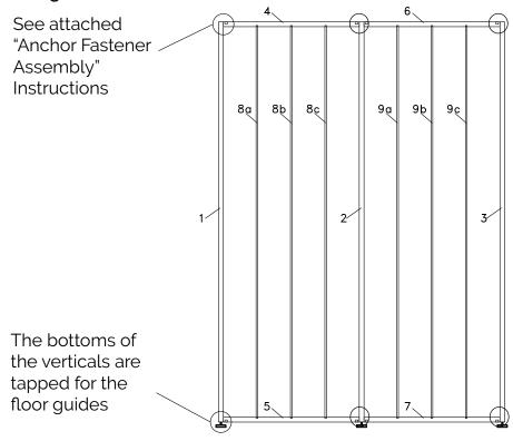
The rods have slots cut for the wood slats to register into.
